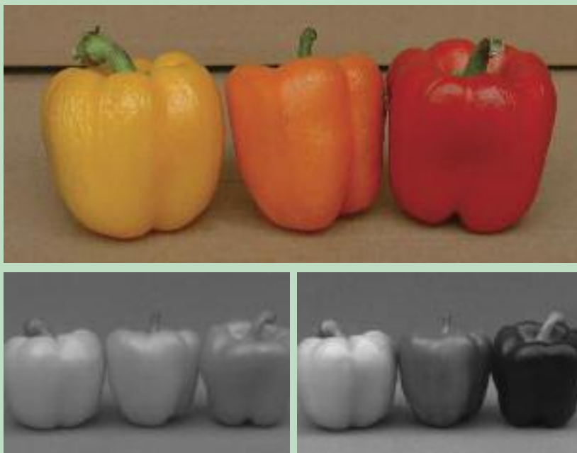
FIGURE 1. To sort bell peppers based on color, different approaches produce very different results. The peppers shown in a photo taken with Fuji digital color camera (top) are then shot with a monochrome camera without a filter and show little contrast (left). A scene shot with the same camera and a BF525 light green bandpass filter shows sufficient contrast for sorting, which is critical given the differing prices of each color pepper (right).
